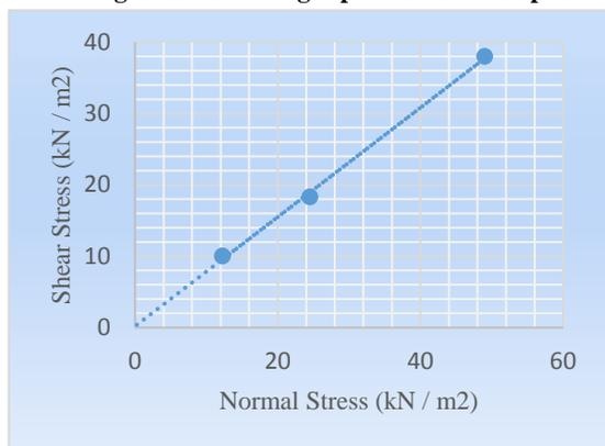
Fig. 9: Shear strength plot for failed slope sample
