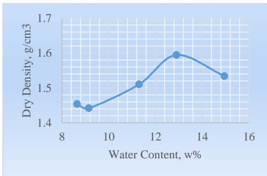
Fig. 5: Maximum Dry Density – Stable Slope
