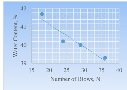
Fig. 1: Liquid Limit Plot – Failed Slope
