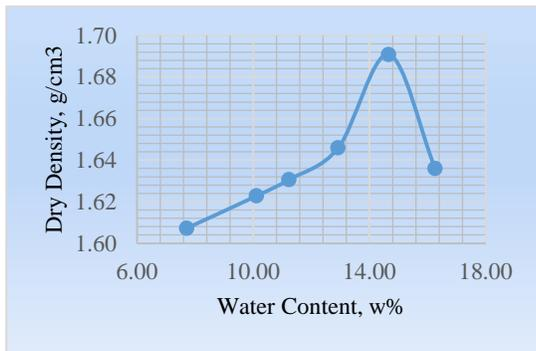
Fig. 2: Maximum Dry Density – Failed Slope
