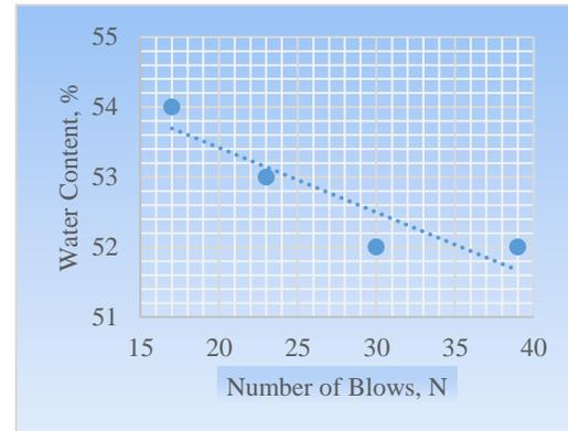
Fig. 2: Liquid Limit Plot – Stable Slope
