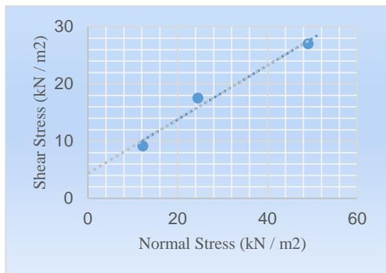
Fig. 8: Shear strength plot for failed slope sample
